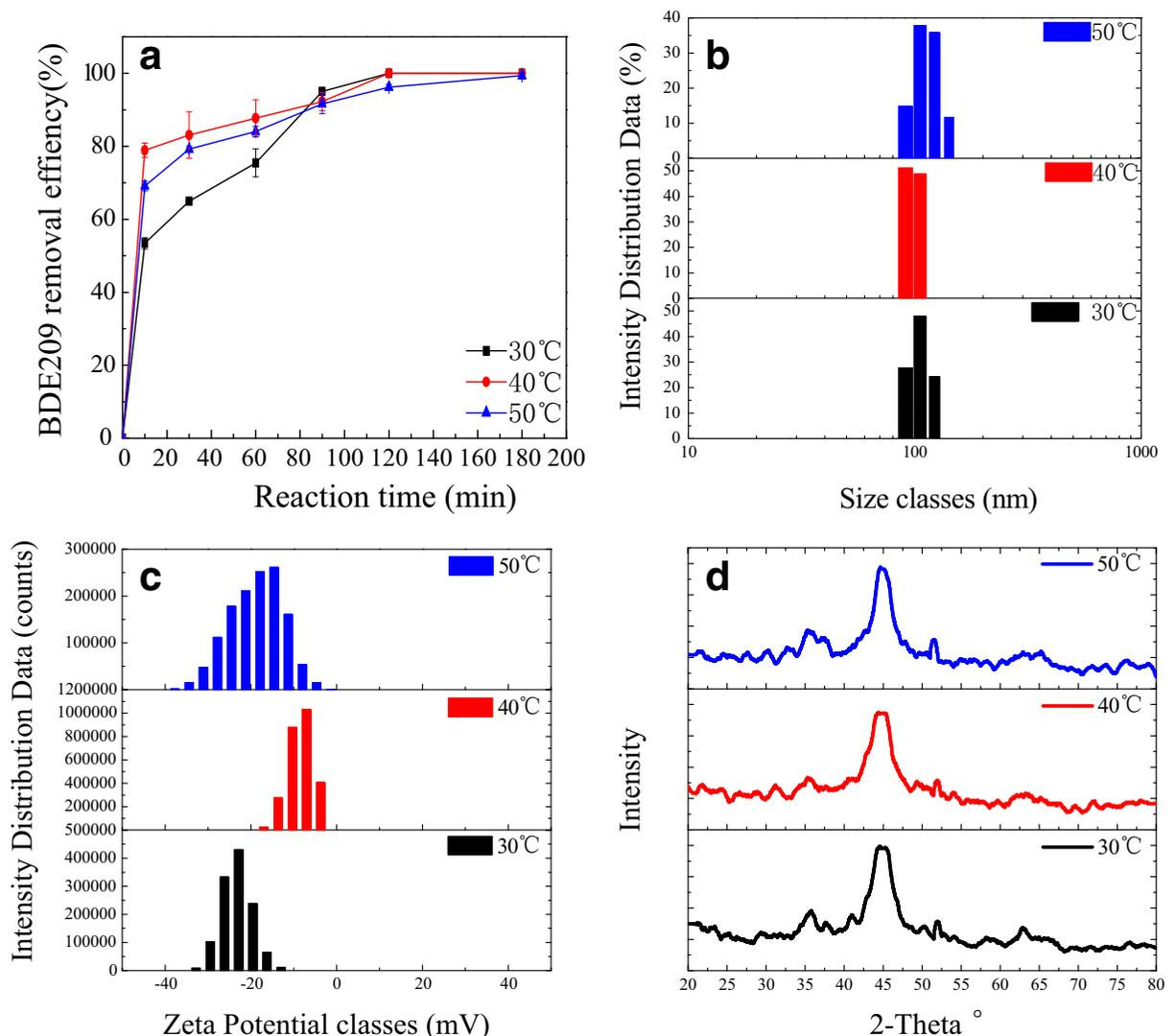
**Fig. 1** Effects of synthesis temperature on the characteristics and reactivity of the Ni/Fe (removal efficiency (a), DLS particle size distribution (b), zeta potential (c), and XRD (d))
