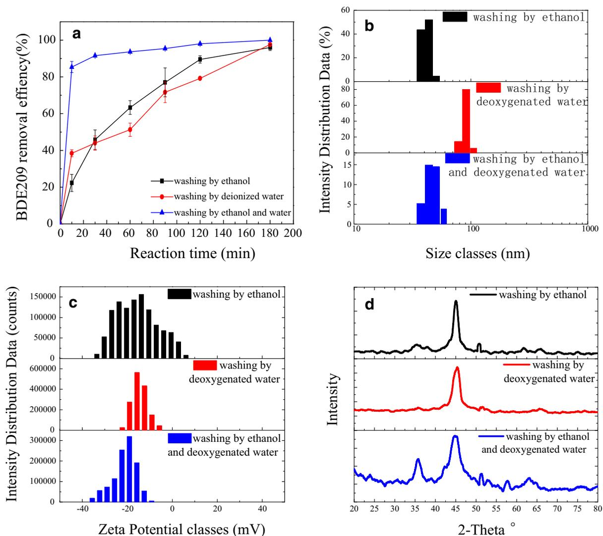
**Fig. 3** Effects of washing solvents on the characteristics and reactivity of the Ni/Fe (removal efficiency (a), size distribution (b), zeta potential (c), and XRD (d))
