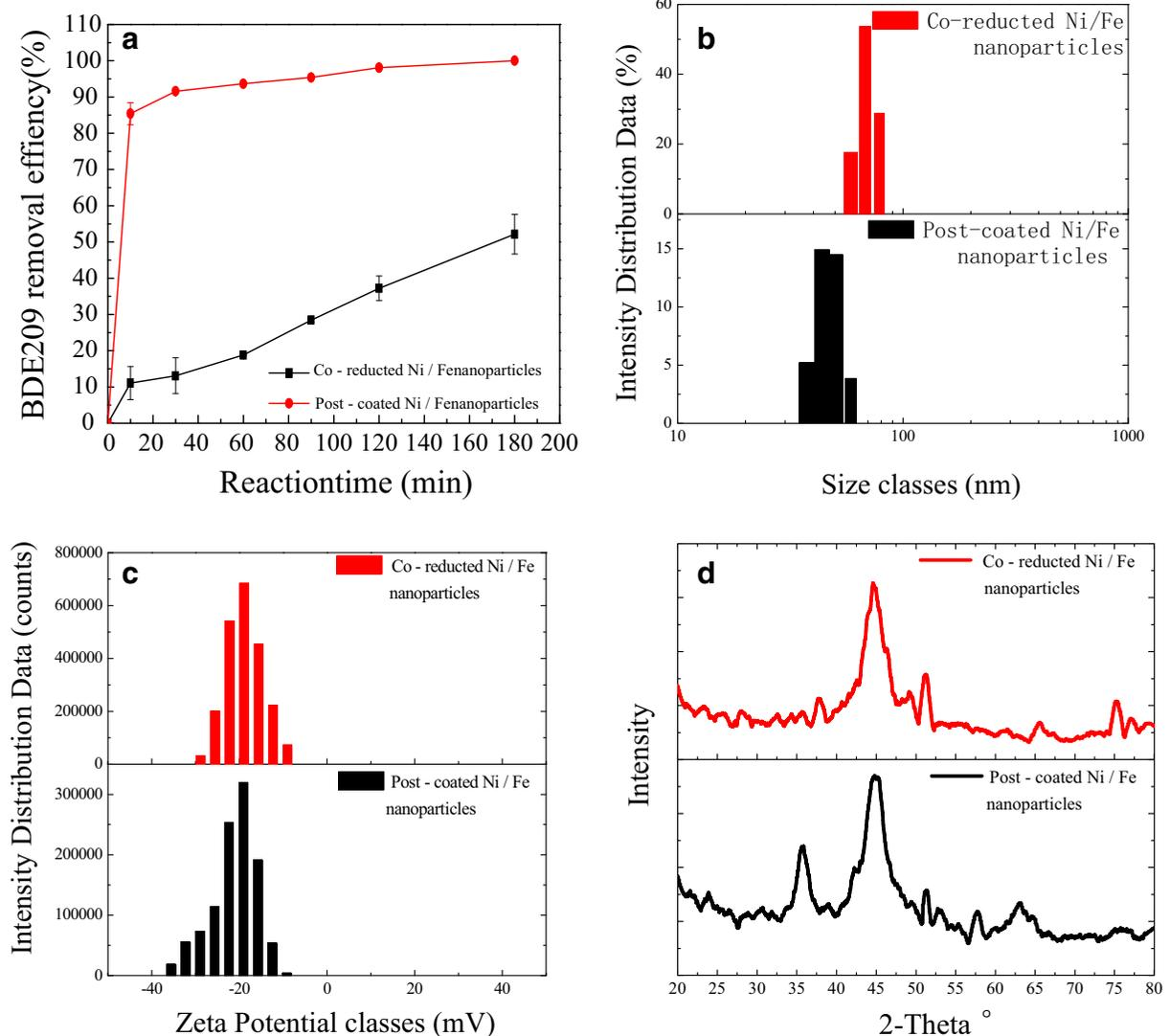
**Fig. 4** Effects of preparing methods on the characteristics and reactivity of the Ni/Fe (removal efficiency (a), size distribution (b), zeta potential (c), and XRD (d))
