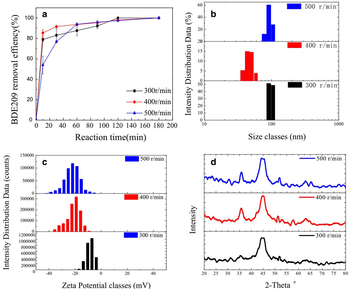
**Fig. 2** Effects of stirring rate on the characteristics and reactivity of the Ni/Fe (removal efficiency (a), size distribution (b), zeta potential (c), and XRD (d))
