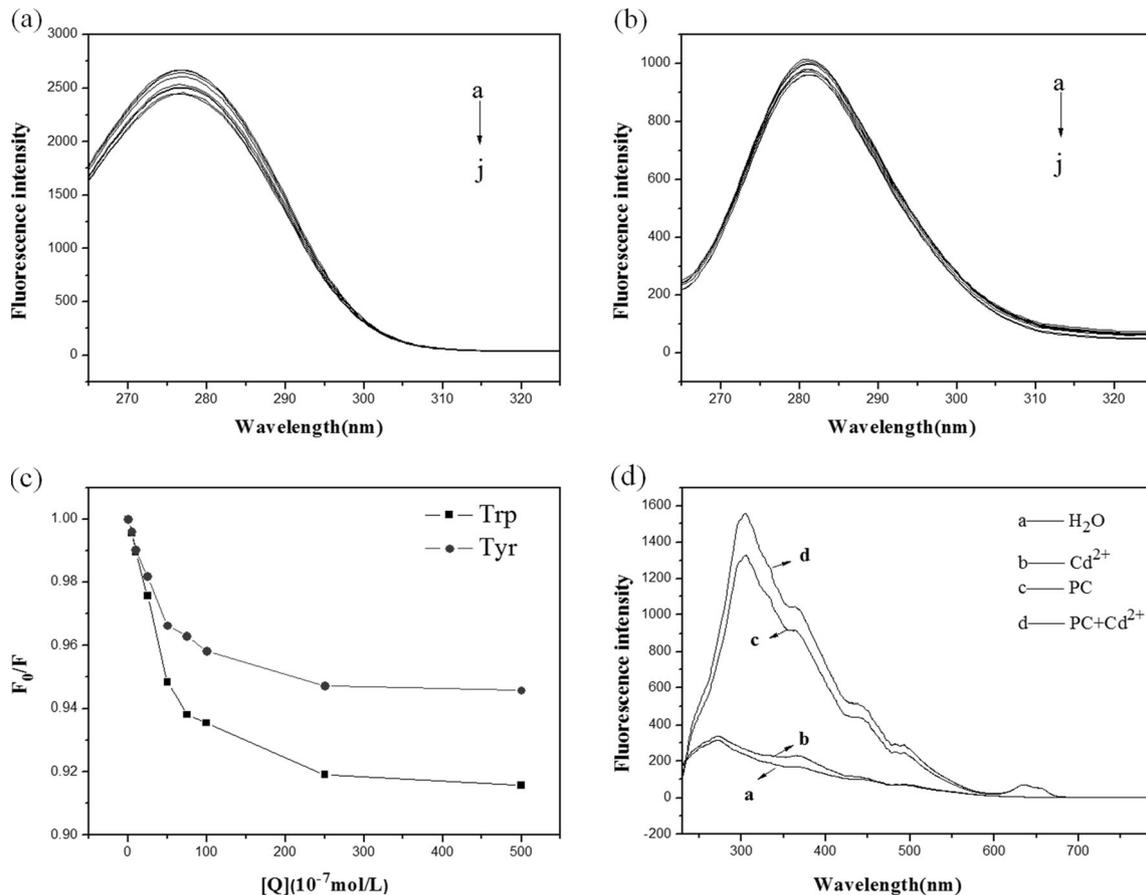
**Fig. 3** Synchronous fluorescence spectra of PC samples with the Cd<sup>2+</sup> concentrations of (×10<sup>-7</sup> mol L<sup>-1</sup>) 0, 5, 10, 25, 50, 75, 100, 175, 250, 450 and 500 (from sub-a to sub-j) at  $\Delta\lambda$  of 60 nm (a) or 15 nm (b); *F<sub>0</sub>/F* plot
