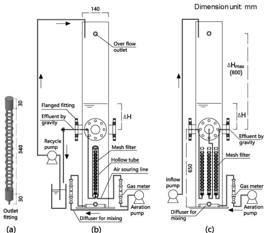
Fig. 1. (a) Frame of the mesh filter, (b) reactor setup for the screening test, and (c) reactor setup for the long-term test.
