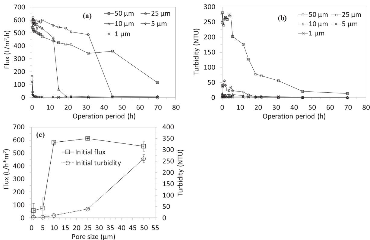
Fig. 2. Changes in the (a) flux and (b) filtrate turbidity for the mesh filters with different pore sizes during the screening test; (c) correlation between initial flux or initial turbidity and mesh filter pore size. Transmembrane pressure = 0.049 kPa, air-scouring strength = 400 mL/min.
