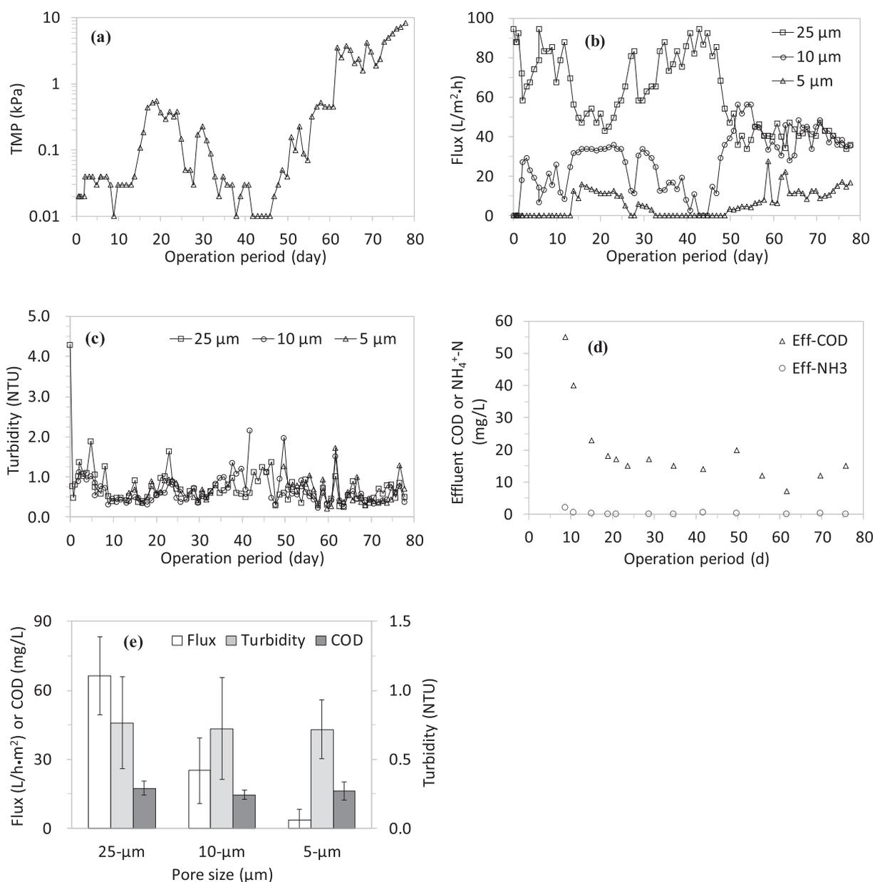
Fig. 3. Changes in the (a) transmembrane pressure (TMP), (b) flux, (c) effluent turbidity, and (d) effluent COD and ammonia concentrations during the long-term test; (e) average flux, turbidity, and COD for the mesh filters with different pore size during the stabilized stage from 2nd to 61st day (TMP = 0.14 ± 0.16 kPa).
